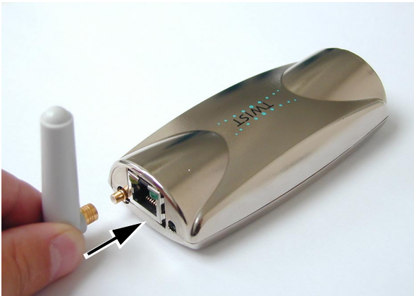
Fig. 3: Installing the GSM antenna
